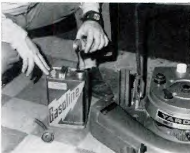
HARD STARTING of two-cycle engine is often the result of not using gas-oil mixture that's specified MARCH 1971
